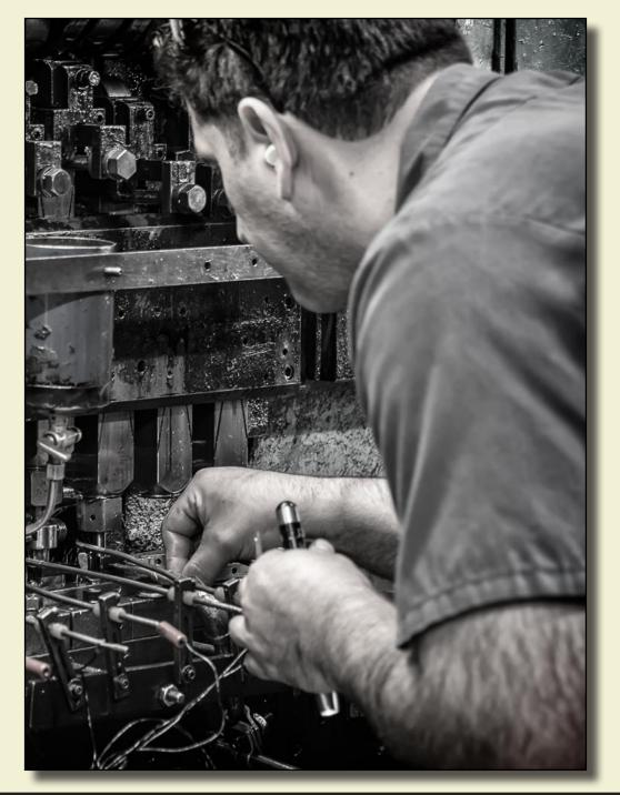
All production, including the **Ziggity** eyelet, begins with coils of flat strip metal. This provides the lowest level of scrap metal loss possible. These custom deep drawn parts are formed as completely as possible within the machine to eliminate and minimize the need for costly secondary operations. The Ziggity eyelet uses stainless steel.
