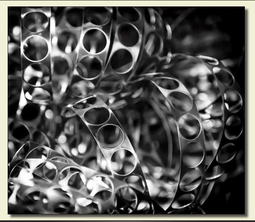
More castoff is created at the end of the press run. Each eyelet gets its final trimming to complete its customer specification requirements.
