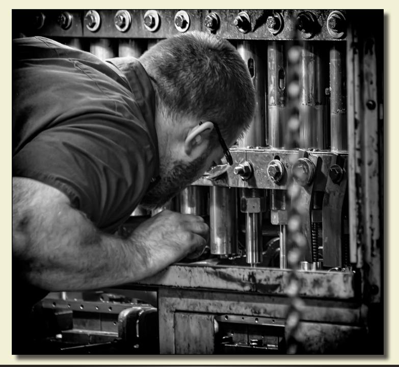
Pete Ulinskas designs any new tool, punches or dies, that the shop may need. As a toolmaker, he works with Mike to maintain the working presses and is also responsible for the setup of any new jobs. He studies blueprints, sketches, models, or specifications to plan operation sequences for fabricating tools, dies, or assemblies; verifies dimensions, alignments, and clearances of finished parts using measuring instruments.
