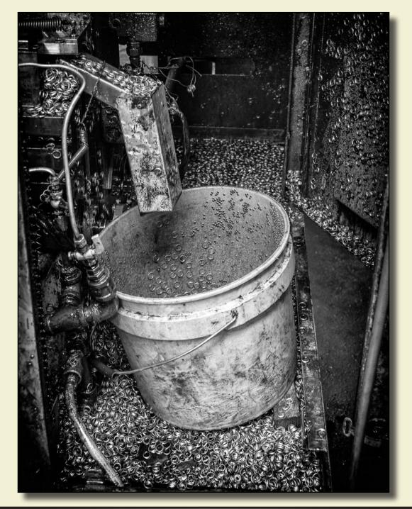
As each production run progresses, completed parts are put into holding buckets for a final visual inspection and is also recorded on inspection sheets. The press operator knows that the parts have met gauge specifications, but must be certain these are visually satisfactory before putting then in the process completed container.
