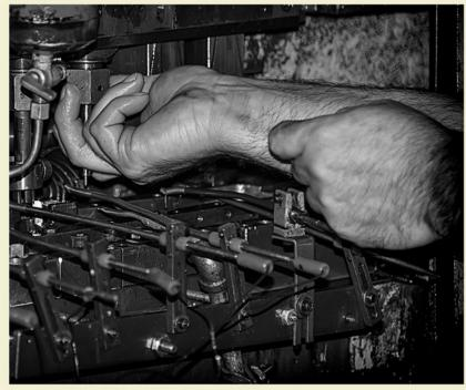
The **Transfer Fingers** of the press move material along its way from one station to the next. Here we see Mike's "fingers in the fingers" as he makes adjustments to the transfer process on the press.
