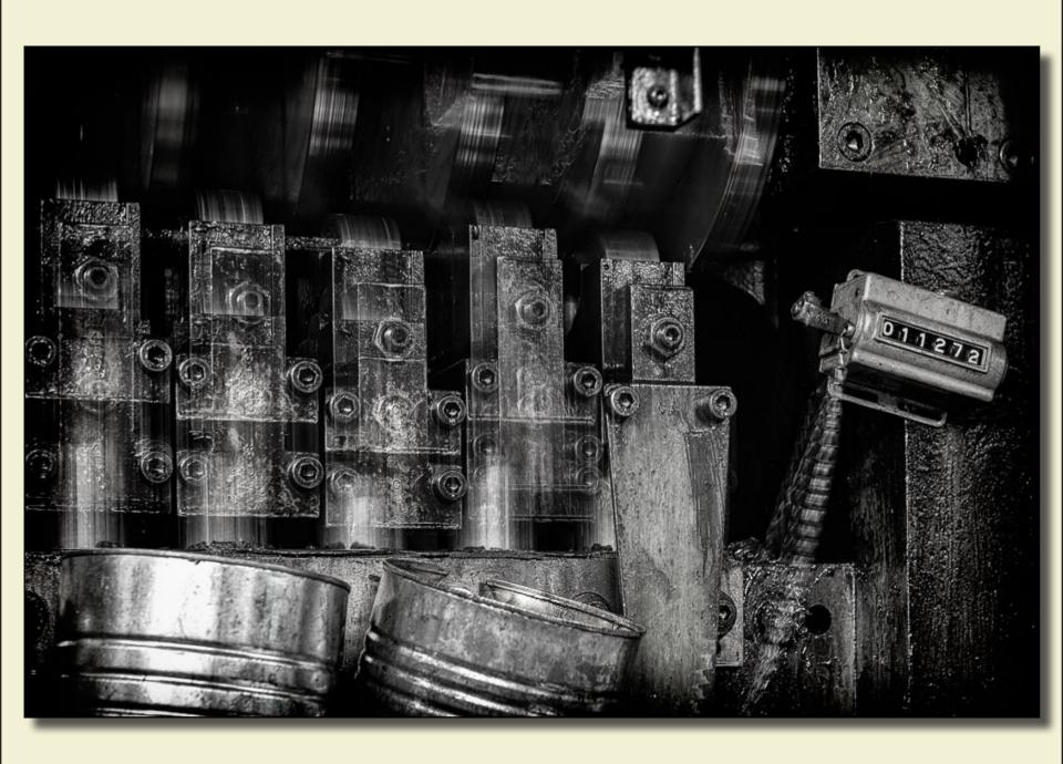
Before the **Ziggity** eyelet begins its transfer journey from stage to stage in the press, the blanking process creates coin-shaped flat material as the starting point. Castoff, or excess material, is created and collected after the blanking to be sold to scrap metal dealers. This helps keep the price of production lower.
