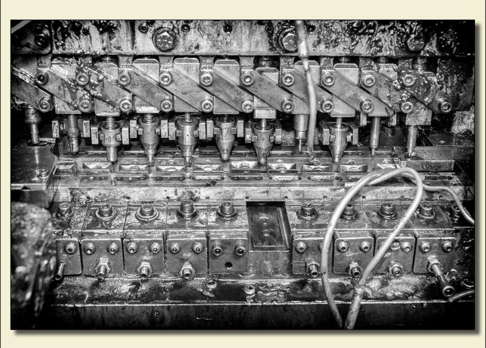
This press is in full operation. Notice the counter keeping score of the day's production run. Approximately 60,000 to 100,000 eyelets are manufactured per day.
