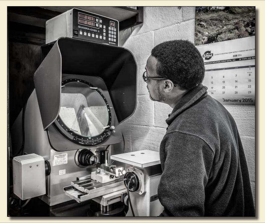
Here is a closer view of the **Comparator** in action. Warren is pointing to the angle on one of the products. The result is compared to the customer requirements and specifications to ensure that these tolerances are met and often exceeded.
