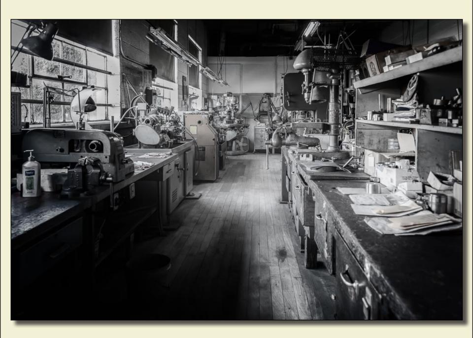
These are speed lathes used for round turning and boring of ID (inner diameter) and OD (outer diameter) of the punches and dies used in each machine press.
