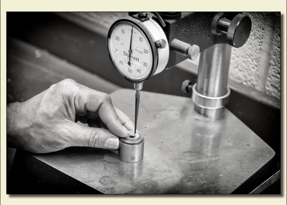
The second machine is called the **Mitutoyo Comparator**. This precision tool is responsible for comparing the radius of various features of the final product to the actual customer order specifications.
