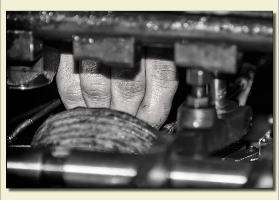
Mike continues to make adjustments to the fingers, punches, dies, as he inspects the general operation of the press before the machine is allowed to resume production. He conducts test runs with completed tools or dies to ensure that parts meet specifications, making adjustments as necessary.
